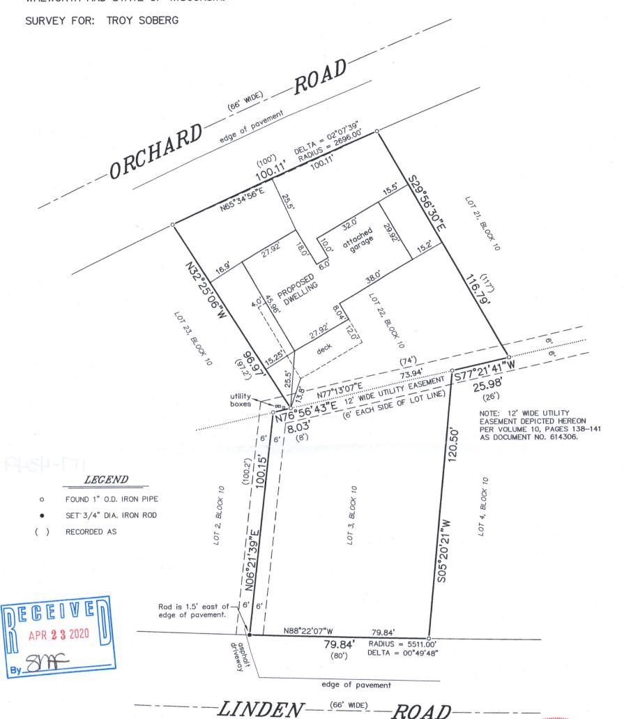
BEARINGS HEREON RELATE TO THE EAST LINE OF LOT 3 IN BLOCK 10 OF WOODDALE ADDITION. ASSUMED BEARING OF SOUTH 05°20'21" WEST TO ORIENTATE WITH A PREVIOUS SURVEY BY J.K. SURVEYING INC. DATED FEBRUARY 15TH, 2005.
